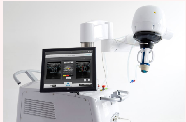
Figure 2: High-intensity focused ultrasound (HIFU) machine
