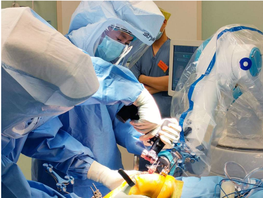
The robotic arm assists the surgeon in executing his bone cuts accurately, according to his surgical plan.
